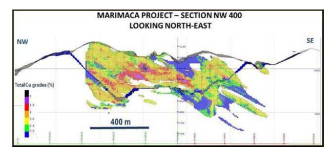
The resources were estimated only for oxide and mixed copper mineralization, which can be processed by heap leaching and run of mine (ROM) leaching to produce cathode copper. No resources were estimated for enriched and primary sulphide mineralization, occurring in deeper portions of the deposit.
