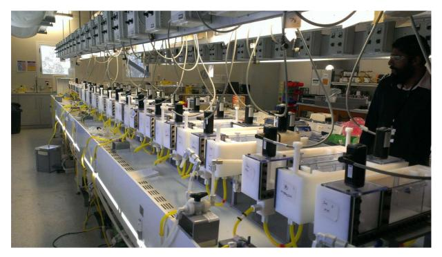
The improvement consisted of the addition of a scrub circuit into the zirconium solvent extraction process, to remove the Hafnium for subsequent refining to produce a saleable hafnium product. This addition was made by the company's team outside of the FEED scope after further research with ANSTO.
