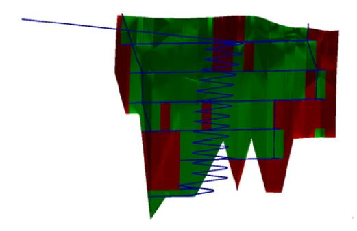
The mining methods would be Long-hole and Shrinkage mining with hydraulic backfill. All underground maintenance and associated services facilities would be located midway of the vertical extent of the known potentially economic mineralized zone. Ventilation would utilize raises at each extremity of the mineralized zones being mined for fresh or return air and the ramp as an exhaust for return air, with a push-pull ventilation arrangement.
