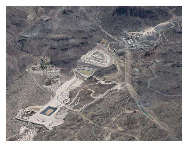
Sufficient mining blocks are available to support a 250 tpd production rate for two years with only minimal development. Three more years of blocks have been estimated but will require development and verification sampling. These blocks have been assayed at an average grade of 7.75 gpt Au with vein widths at 1.5 to 1.8 meters. The mine has been dewatered, electrical power and compressed air are available at all levels and the ventilation system fans have been re-installed.
