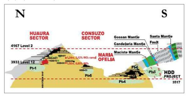
The mine consists of three sectors, Consuzo, Huara and Huayllapon. These are shown on the crosssection above. The only
