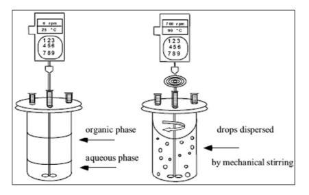
In the first instance the imprint molecule is dissolved in an organic matrix, including monomers and initiator. Then there is a secondary aqueous phase that provides surfactants and thermal dampening. Then shear and heat applied to form droplets of desired size that polymerize and harden into beads.
