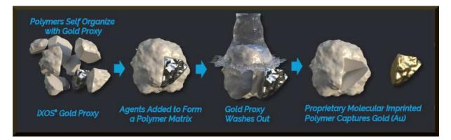
Below is another representation of the process. In some ways this strikes us as being the chemical equivalent of the Lost Wax Process used in casting:
