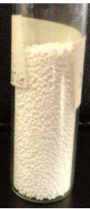
With gold mining, the bead technology has the potential to replace the current Carbon-in-Leach (CIL) material which is now used in about 500 operating gold mines. A prime attraction is that mines will not have to do any retrofit or significant process changes, instead they essentially replace the carbon with the polymer beads.
