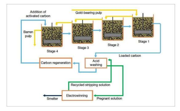
Carbon-in-pulp (CIP) is an extraction technique for recovery of gold which has been liberated into a
