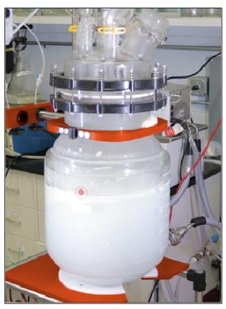
suspension to form beads. Adjustments in the suspension, mixing rate, and addition rate of the monomers are done to get a bead of the size and porosity that are optimal for the desired applications.
