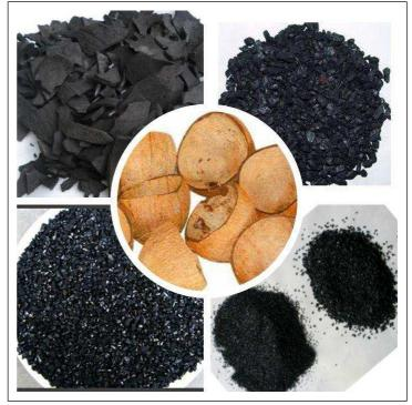
(GCP). For suitable GCP solutions activated carbon is the most common sequestering substrate for the removal of dicyanoaurate, accounting for over half of all gold extracted.
